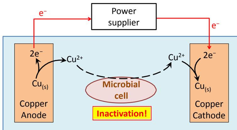
Fig 1. Illustration of electrochemical disinfection.  $\text{Cu}^{2+}$  released at the anode inactivates microorganisms. Simultaneously,  $\text{Cu}^{2+}$  is recovered as metallic copper at the cathode
